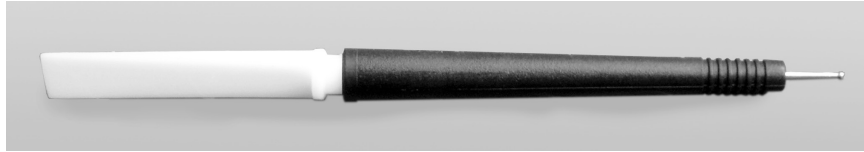
Figure 2. Huffman used a spring-loaded ball burnisher similar to this one.
